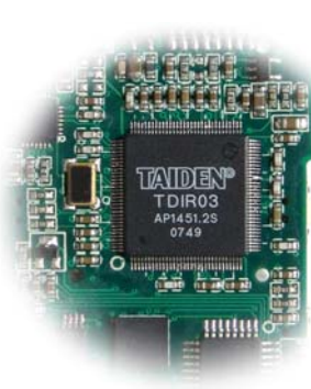
Figure 1 TAIDEN TDIR03 digital infrared processing chip
