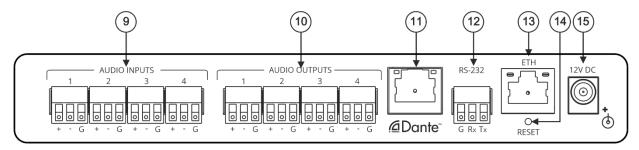
Figure 2: FC-404NETxI 4x4 Audio and Dante Mixer Front Panel
