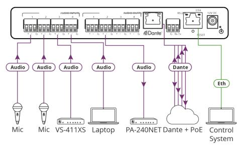
Figure 3: Connecting to the FC-404NETxl Rear Panel
