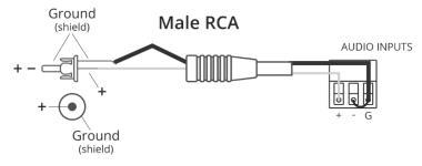
Figure 6: Connecting an Unbalanced RCA Input
