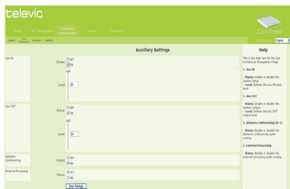
Activating the external processing allows to add external signal processing equipment or a mixing board.
