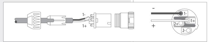
Connect the positive wire (amplifier '+' output) to the pin 1+ of the SPEAKON connector. Connect the negative wire (amplifier '-' output) to the pin 1- of the SPEAKON connector. The pins 2+ and 2- are not used.
